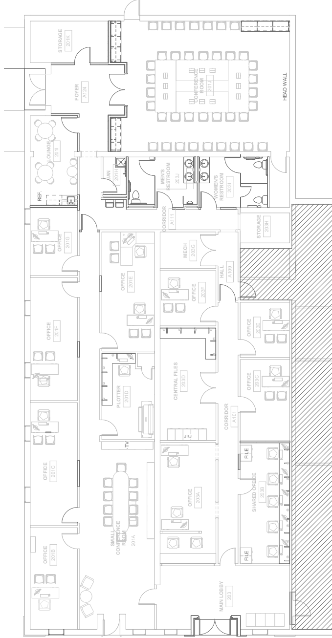
① FURNITURE LAYOUT PLAN 3/16" = 1'-0" NOTE: FURNITURE BY OTHER, UNLESS OTHERWISE NOTED OR DETAILED
